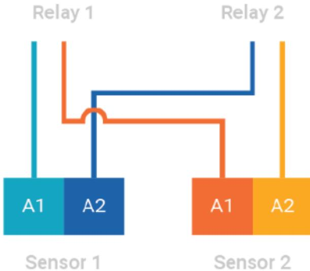
Discrete mode allows a separate action for each sensor. Relay 1 is actuated by Sensor 1 alarms and Relay 2 is actuated by Sensor 2 alarms
