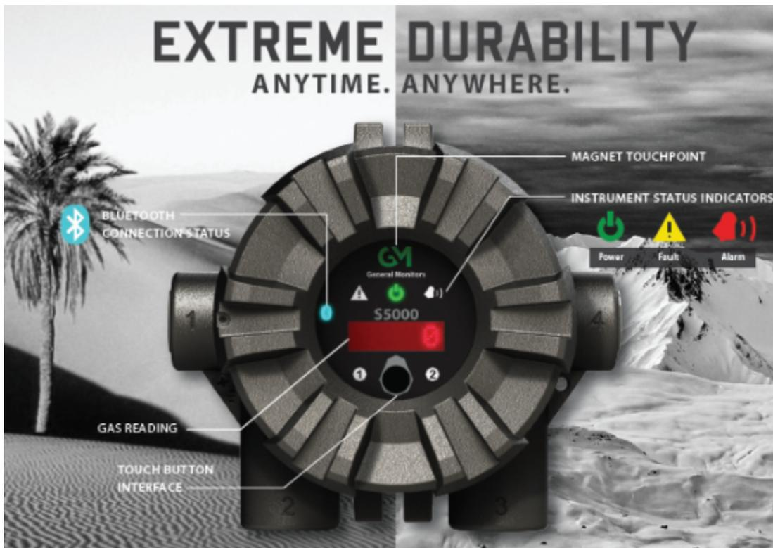
In addition to the red LED display, the S5000 uses six icons to indicate status. Green LED indicates power supply status. A yellow triangle and red bell indicate fault and warning or alarm conditions respectively. The Bluetooth<sup>®</sup> icon indicates that the Bluetooth<sup>®</sup> wireless technology is enabled on the device. Yellow "1" and "2" icon indicate which sensor gas reading is being displayed, or during configuration which sensor's options are being accessed.
