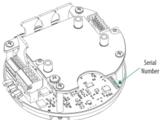
Figure 6 Digital Sensor - Position of Labels
