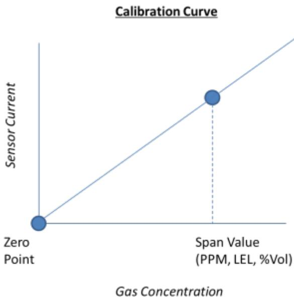
The Sensor Span Value (i.e. Cal Level) in the device menu should be the same as the concentration listed on the calibration gas cylinder.
