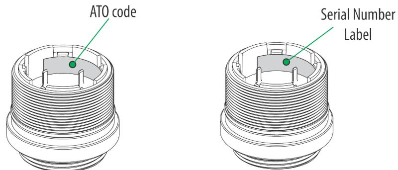
Figure 7 IR Sensor - Position of Labels
