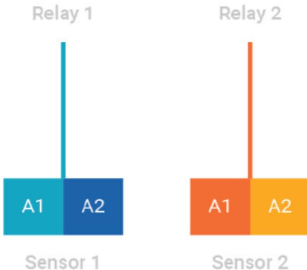
Horn mode is designed to allow local acknowledgment of a relay-triggered horn, while the alarm state is still present. All alarms on both sensors trigger both relays, however the second relay can be acknowledged through the "Reset" entry in UI menu by touching the EZ touch button or applying magnet to the GMI logo.
