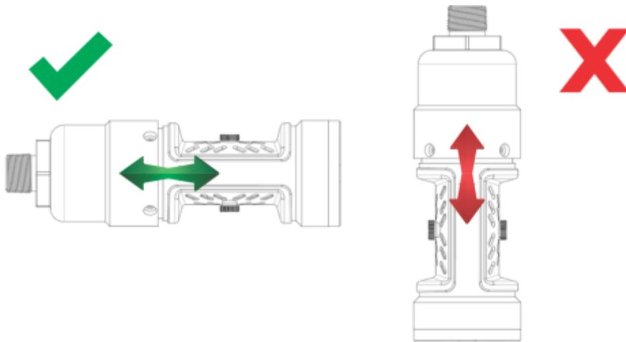
All other sensors, including electrochemical, catalytic bead, oxygen, passive catalytic bead, and passive MOS should be mounted vertically with the gas inlet pointed downward. If the sensor is not mounted with the gas inlet facing down, it is more likely to become clogged with particulate matter or liquids. Figure 11 shows the correct and incorrect mounting orientation for digital sensors. Passive catalytic bead and MOS sensors come already installed on the transmitter housing.
